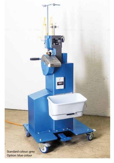
The Dohle stand-mounted machines are equipped with a sliding wheel with pins for easy fabric transport.
